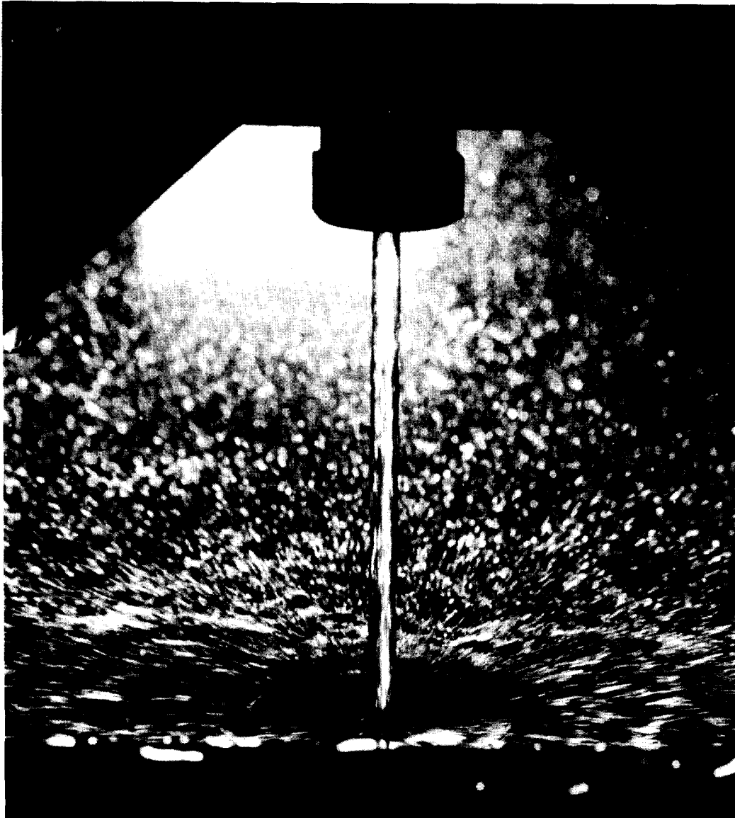
Figure 7. Liquid jet impacting slightly concave plate (69 kPa gauge delivery pressure, 2.54 cm plate diameter, 1.87 cm nozzle to plate spacing, 1/18,000 s flash duration).
