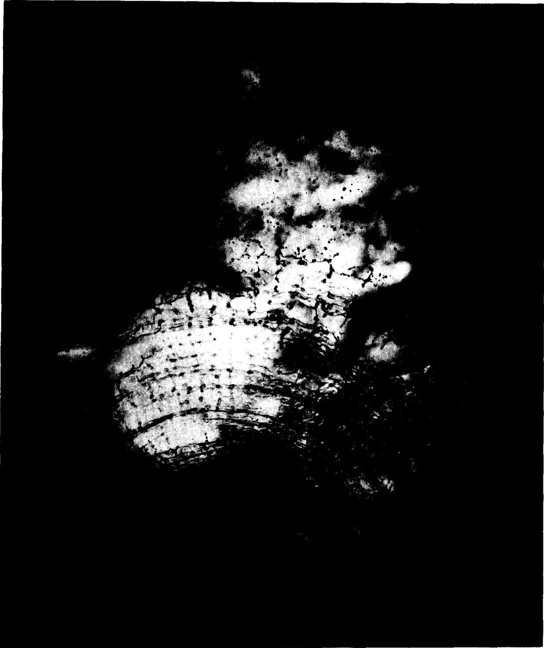
Figure 9. Liquid fan sheet breakup into drops (110 kPa gauge delivery pressure, 1.90 cm plate diameter, 1.87 cm nozzle to plate spacing).
